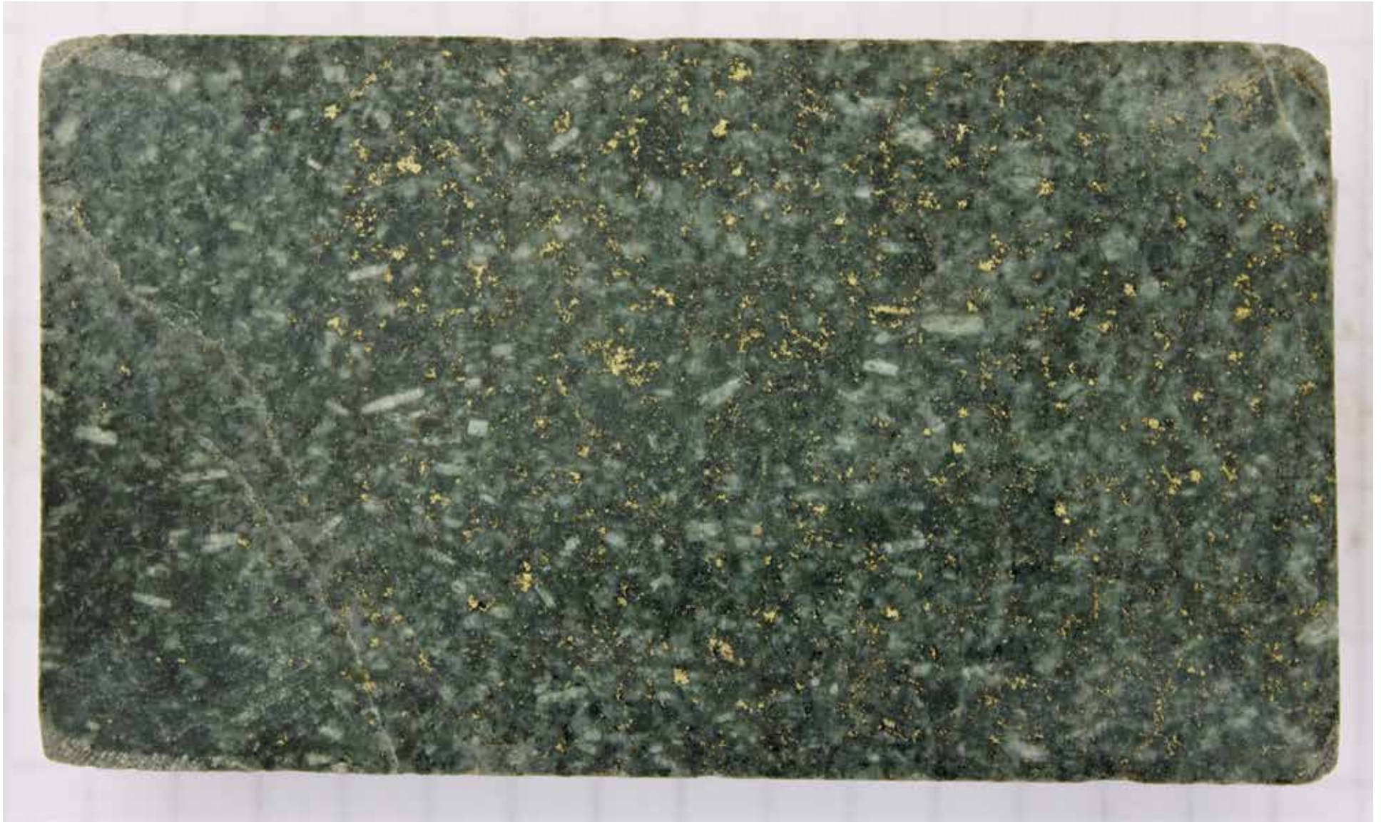
Iron Cap zone – fine grained porphyry with and kspar alteration, disseminated sulfides
