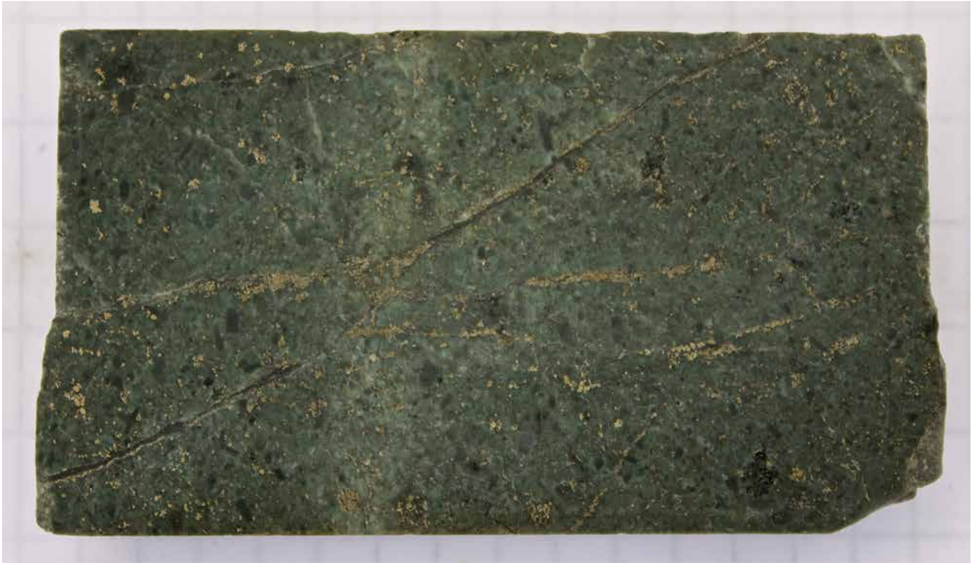
Sulphurets zone - fine grained, inequigranular; chlorite and kspar alteration, dissem. and veinlet sulfides
