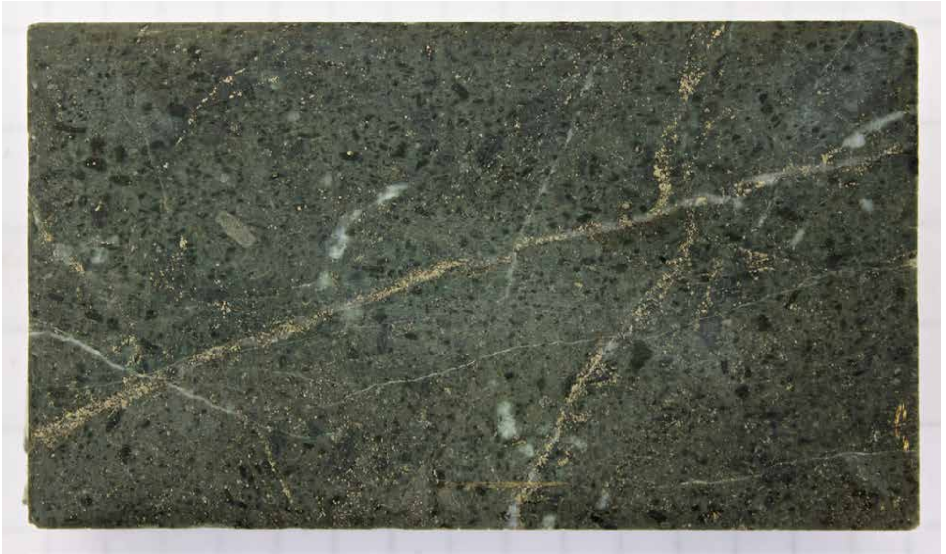
Kerr zone – fine grained, porphyritic, chlorite and kspars alteration, disseminated and veinlet sulfides
