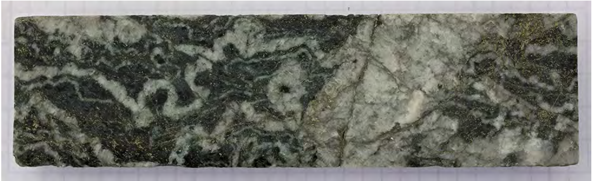
Mitchell zone – polyphase deformed, crackled stockwork qtz veins, dissem. py, cpy, Au, kspar-mt altn.
