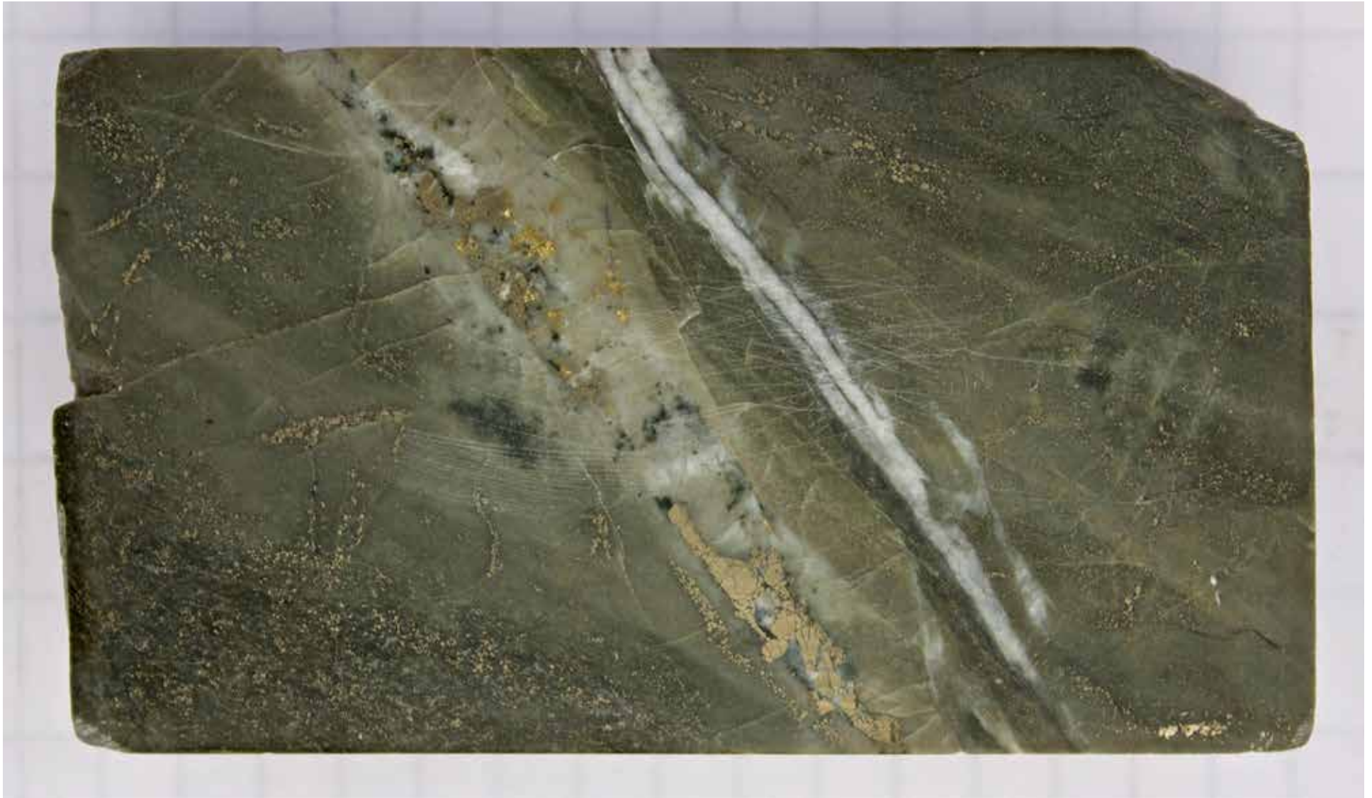
Camp zone – silicified micrite with py-Au vein, silica selvage, late parallel carb vein.
