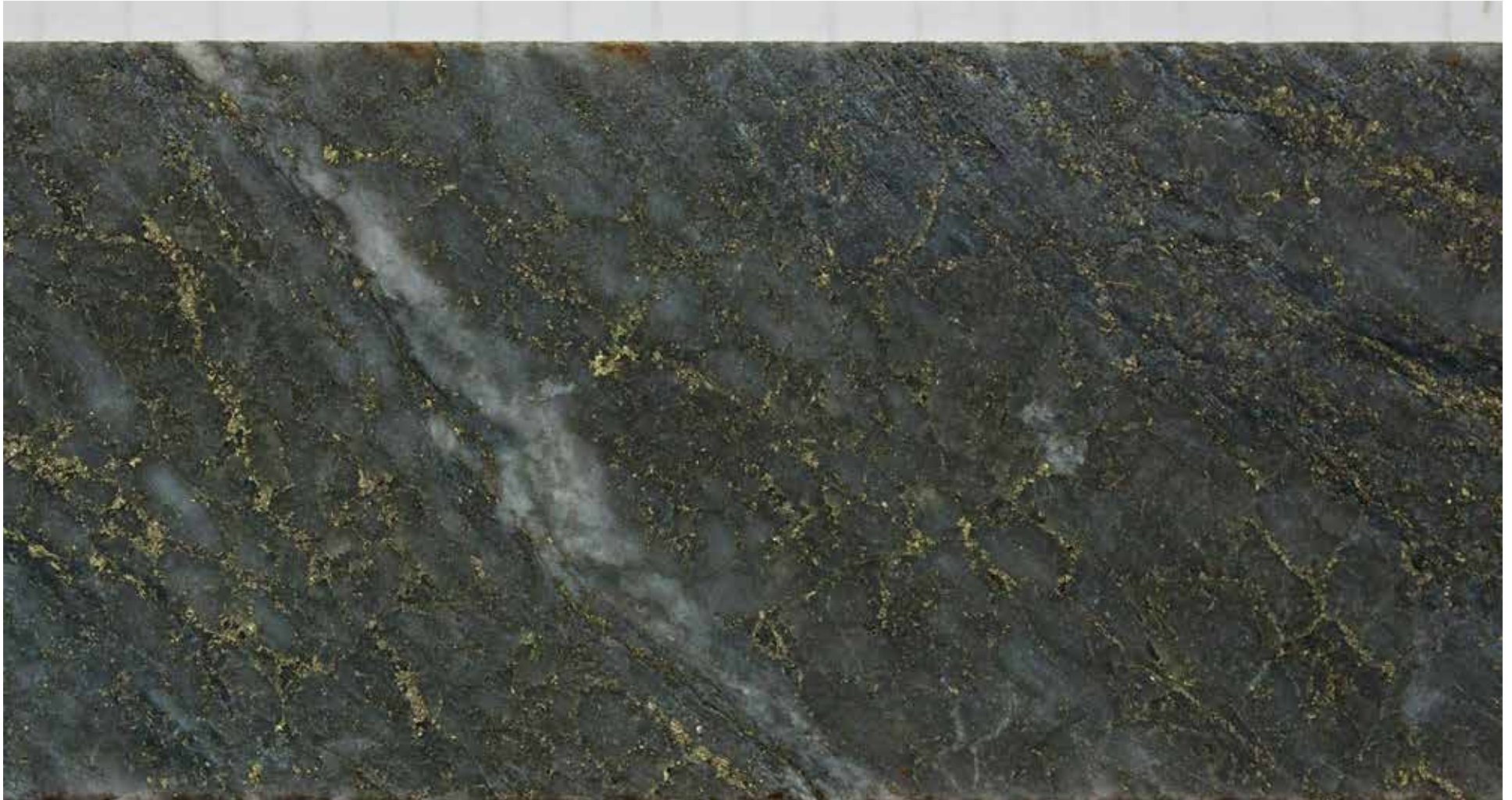
Kerr zone – silicified wall rocks with crackle and diss. cpy, born, Au
