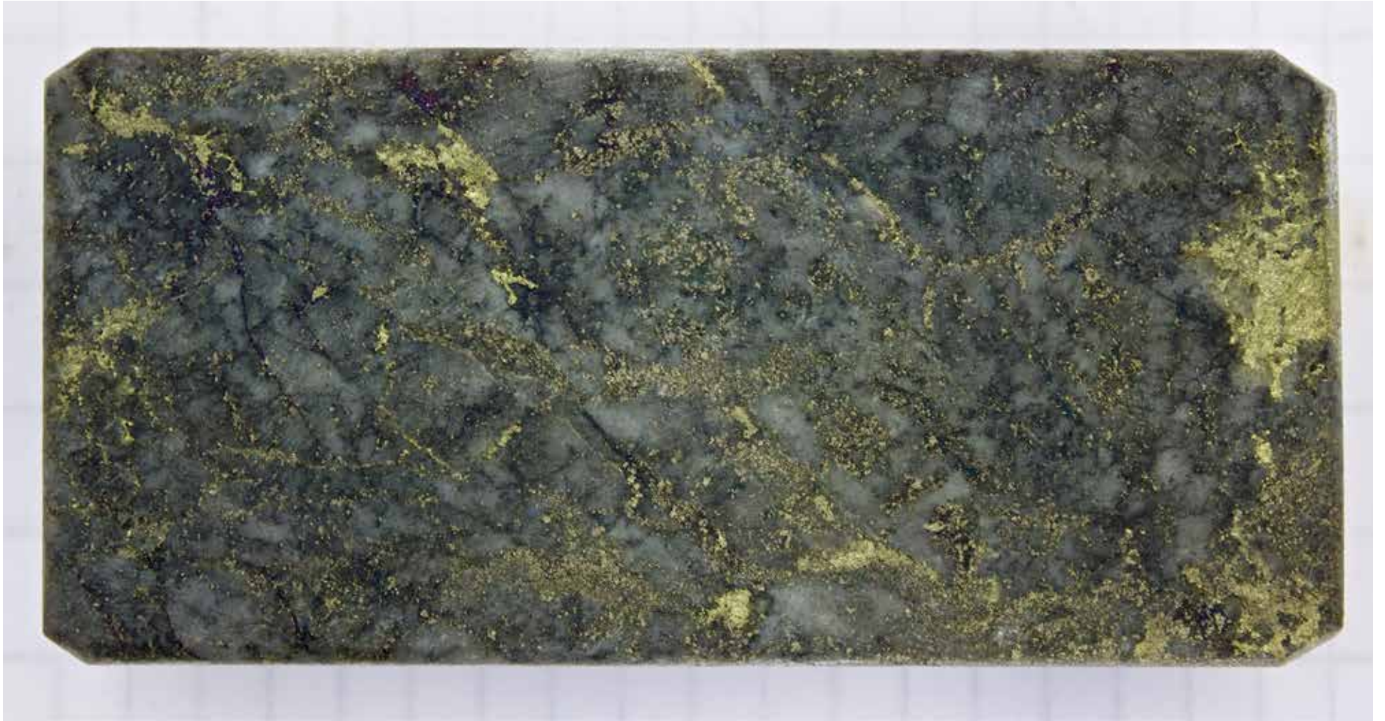
Kerr zone – sheared, crackled qtz vein with cpy, born, Au
